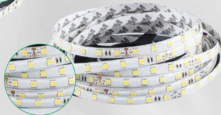
LED strip 24V, 60 diodes 5050 SMD per meter 14.4W/r.m., waterproof IP65
